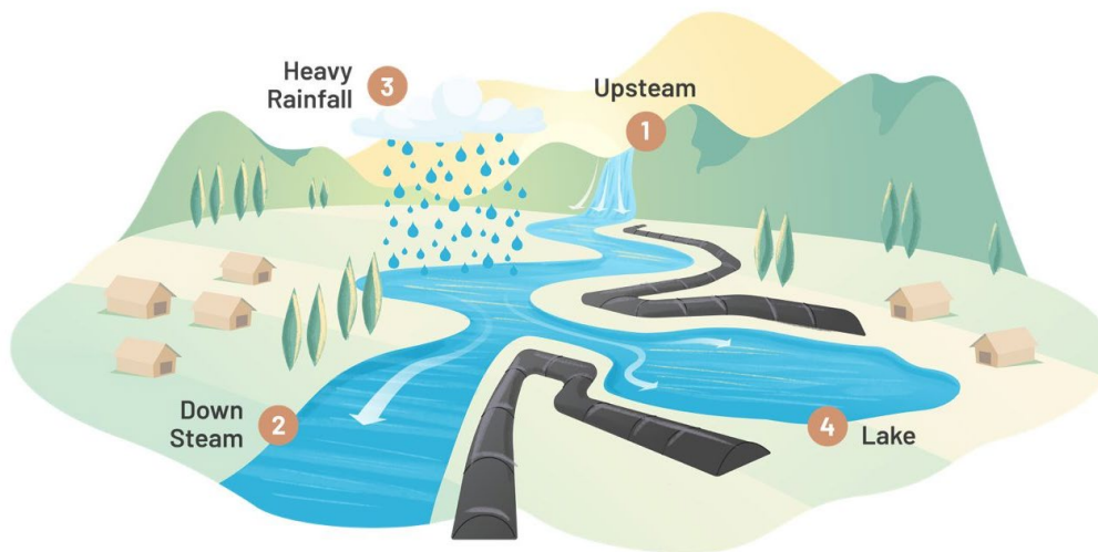
Figure 7: Water-filled flood barrier will serve as a water harvesting infrastructure
